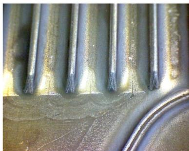
**Figure 20. Formed samples in coated 441, 0.5 mm**
