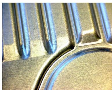
**Figure 19. Formed samples in coated 441, 0.3 mm**
